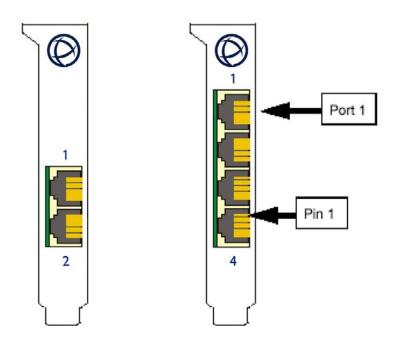
The RJ45 connector has a 10-pin configuration. If you require an 8-pin connector configuration, use the pinouts in the RJ45 8-pin column. The connector pinout for each RJ45 socket fitted to the SPEED LE cards is as follows;
